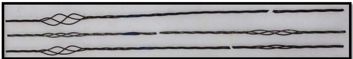
Figure-6: Failure modes of STARK Steel
